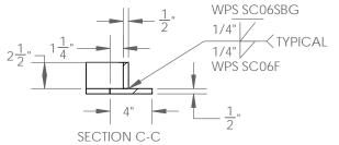
1.) ALL MATERIAL SHALL BE HOT ROLLED STEEL CONFORMING TO THE REQUIREMENTS OF ASTM A709 GR36 (A36).
